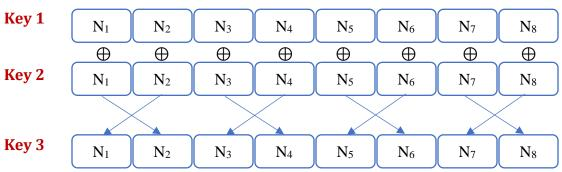
So basically, the first key and the second key are XORed with each other. The nibbles are swapped in each byte and stored in the third key.
